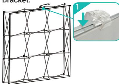
**a.** Snap the LED Light Bracket on top of the frame. Then slide the LED Light onto the bracket.
